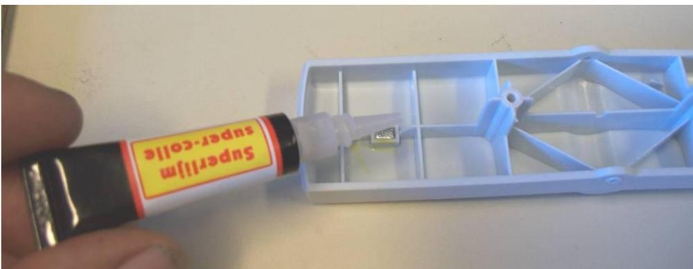
Foto 5 Gluing in the magnet
